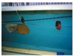
This system works well since you would be sitting on the low side and would want the traveler to move toward the high side. The idea behind the windward-sheeting traveler is to be able to point higher, especially in lighter air, by keeping the boom on the centerline or even to windward a little bit. This helps the boat to point in conditions that pointing is otherwise difficult.
